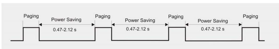
Figure 33: Power saving and paging in GSM networks
