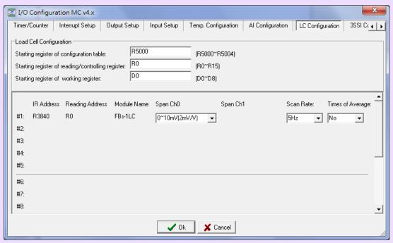
Before FBs-1LC module can be working, the configuration of the module should be set by the Winproladder software tool. The picture shown at above is the I/O configuration page for "LC module" setup.
