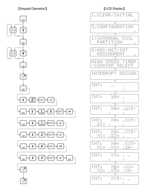
• External interrupt shares the 16 high-speed input points, X0~X15, with HSC and SPD instructions. Therefore, the number of the input points used by HSC or SPD cannot configure for external interrupt.
