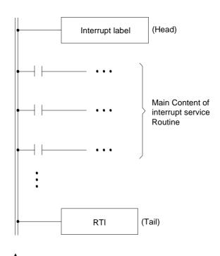
The power line for subroutine is indicated bydouble lines to differentiate from the power line for the main program (single line) for easy reading.
