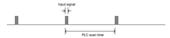
The FBs series PLC main unit supports the captured input function as mentioned above, except this, it also supplies the digital filtering function for digital inputs  $X0\sim X35$ . There are 6 groups of digital inputs  $\{(X0\sim X3)\cdot(X4\sim X7)\cdot(X8\sim X11)\cdot(X12\sim X15)\cdot(X16\sim X23)\cdot(X24\sim X35)\}$  for filtering setting.
